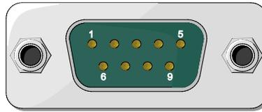
Figure 9: COM port diagram
