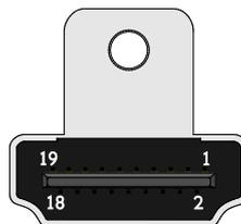
Figure 8: HDMI® port diagram
