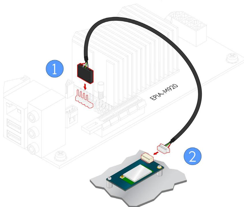
Figure 79: Connecting the USB Wi-Fi cable (VIA EMIO-5531)
