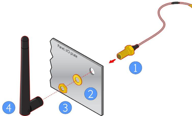
Figure 76: Installing Wi-Fi antenna cable (VIA EMIO-1533)
