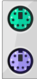
Figure 7: PS/2 port diagram
