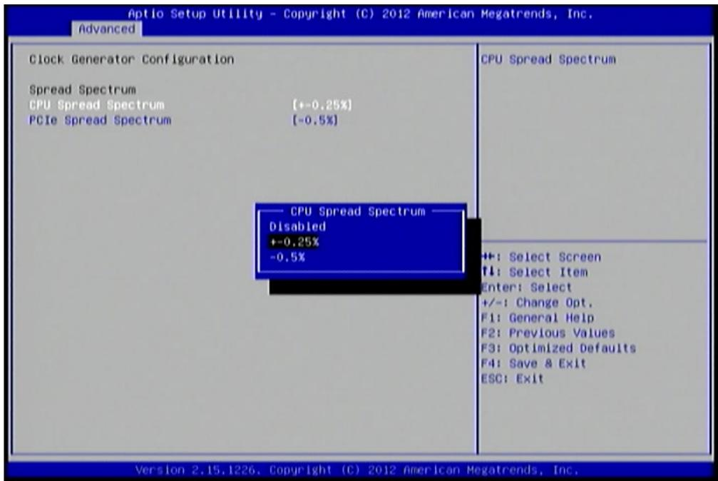
Figure 60: Illustration of Clock Generator Configuration screen
