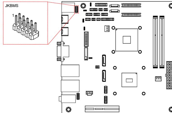
Figure 26: PS/2 keyboard and mouse pin header diagram
