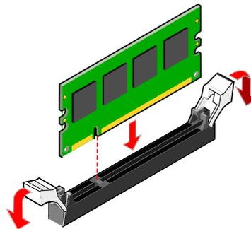
Figure 43: Inserting the memory module
