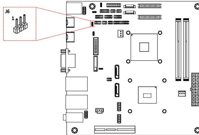
Figure 38: SPI address jumper diagram
