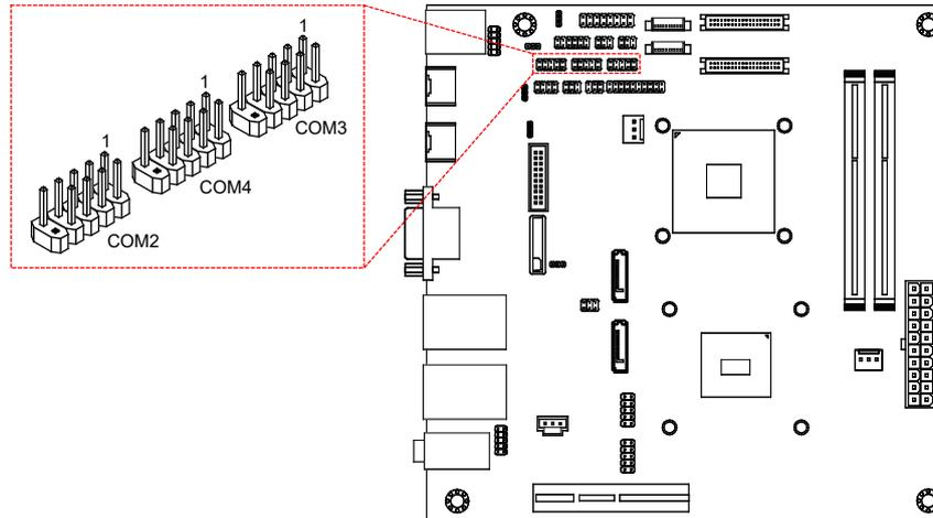
Figure 25: COM pin header diagram
