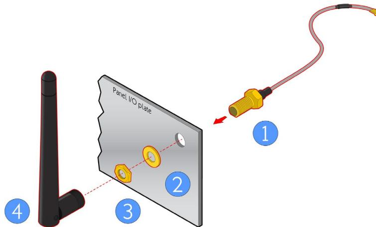
Figure 80: Installing Wi-Fi antenna cable (VIA EMIO-5531)
