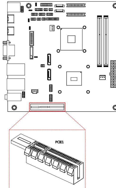
Figure 47: PCI Express slot diagram
