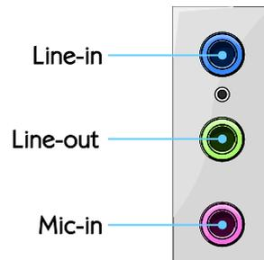
Figure 11: Audio jack receptacle stack
