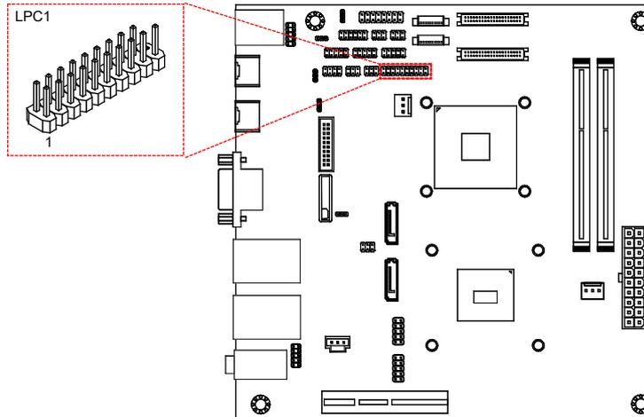
Figure 29: LPC pin header diagram
