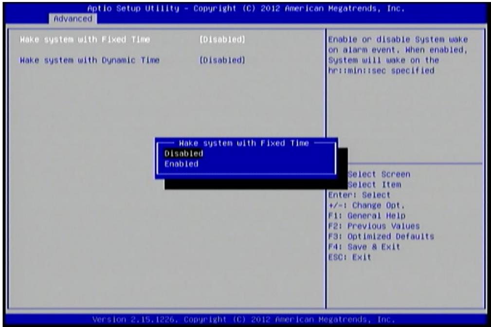
Figure 55: Illustration of S5 RTC Wake Settings screen
