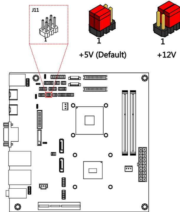
Figure 36: COM1 and COM2 voltage jumper diagram
