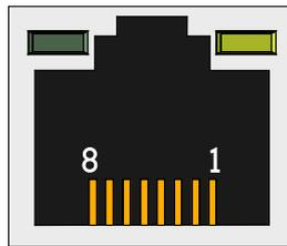
Figure 10: Gigabit Ethernet port diagram
