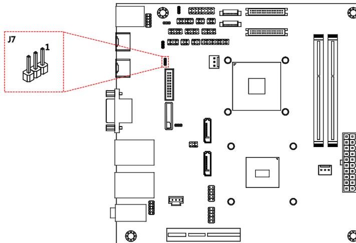
Figure 19: External thermal resister pin header diagram
