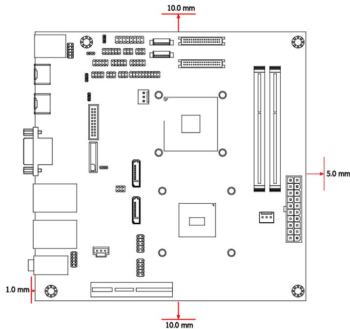
**Figure 48: Suggested minimum chassis dimensions**
