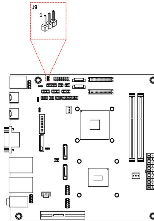
Figure 39: VDD power jumper diagram
