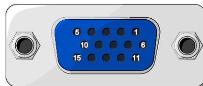
Figure 12: VGA port diagram
