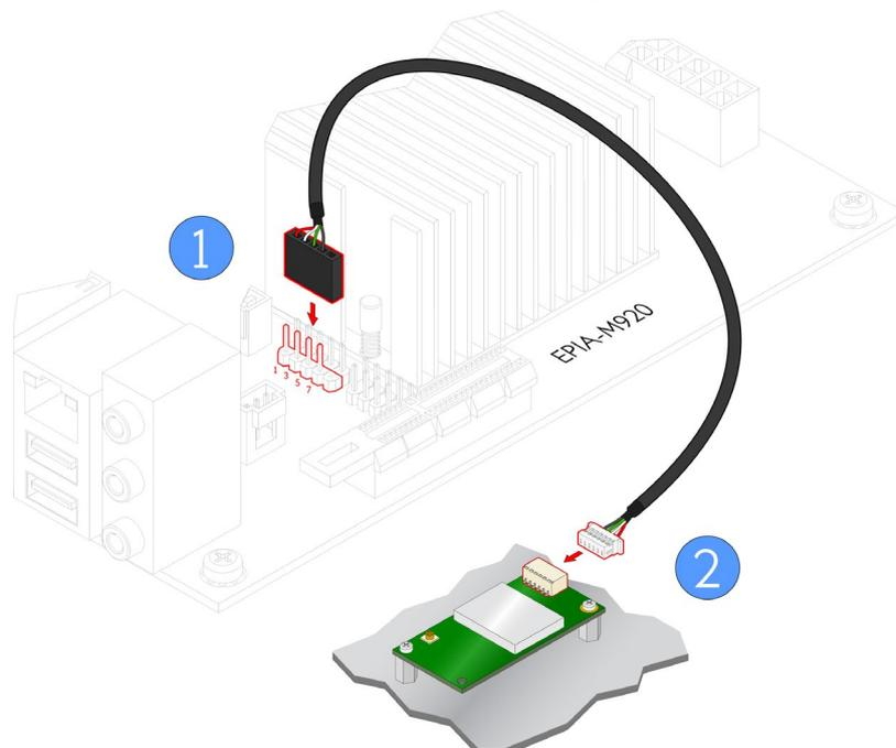
Figure 75: Connecting the USB Wi-Fi cable (VIA EMIO-1533)
