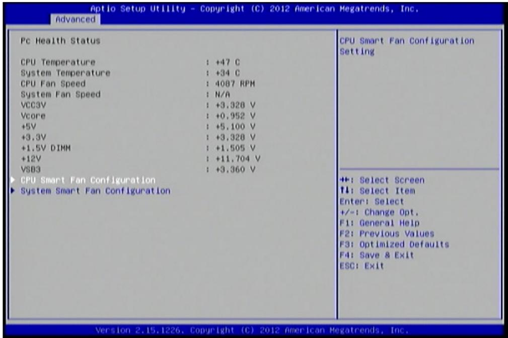
Figure 59: Illustration of F71869 H/W Monitor screen
