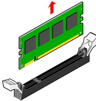
Figure 46: Removing the memory module
