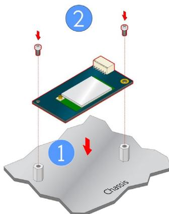
Figure 78: Installing VIA EMIO-5531 module to the chassis
