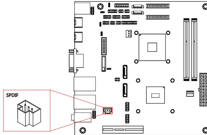
Figure 30: S/PDIF connector diagram
