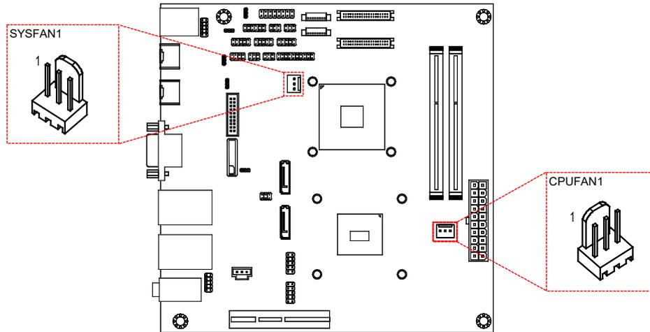
Figure 22: CPU and System fan connector diagram
