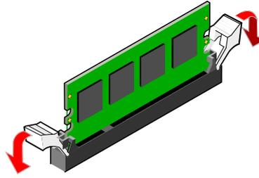
Figure 45: Disengaging the locking clips
