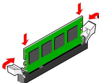
Figure 44: Locking the memory module
