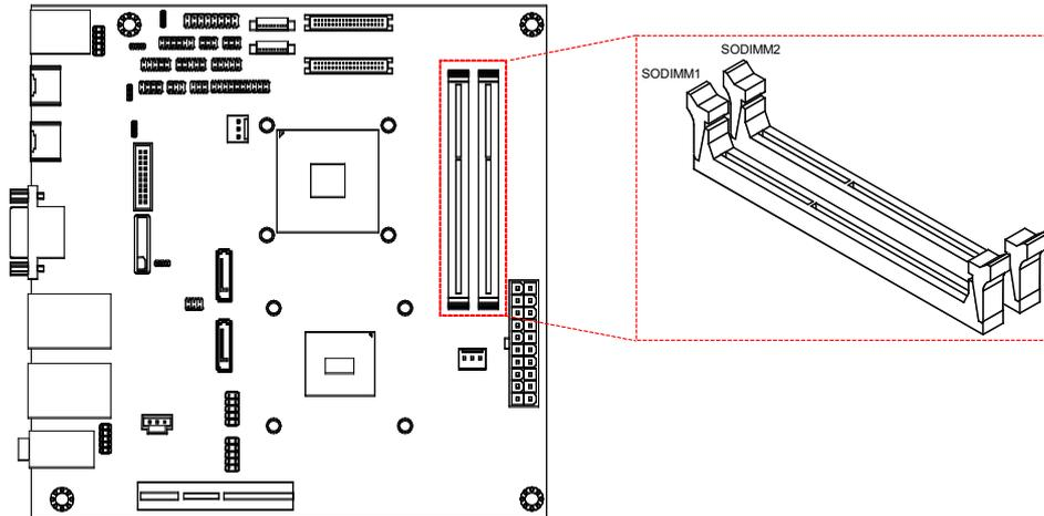
Figure 42: DDR3 memory slots diagram
