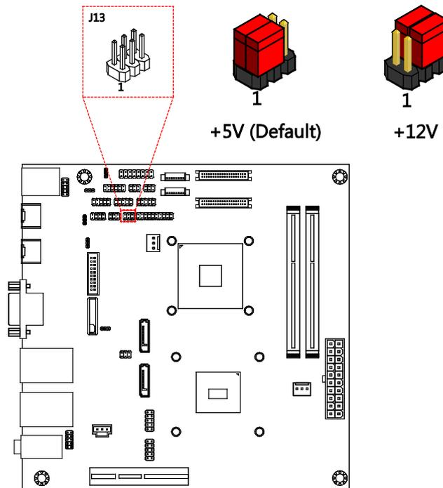
Figure 37: COM3 and COM4 voltage jumper diagram
