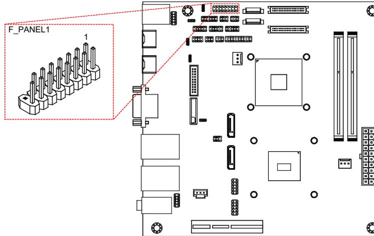
Figure 20: Front panel pin header diagram
