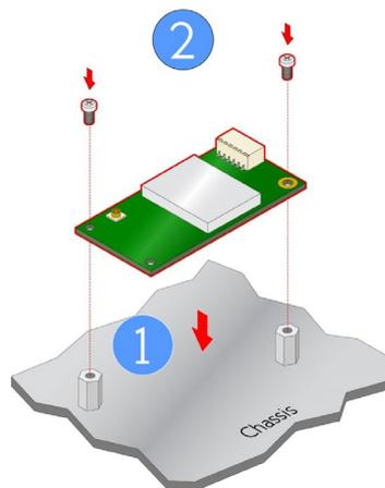
Figure 74: Installing VIA EMIO-1533 module to the chassis
