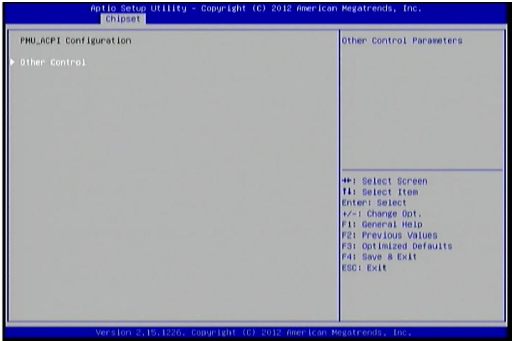
Figure 66: Illustration of PMU\_ACPI Configuration screen Other Control
