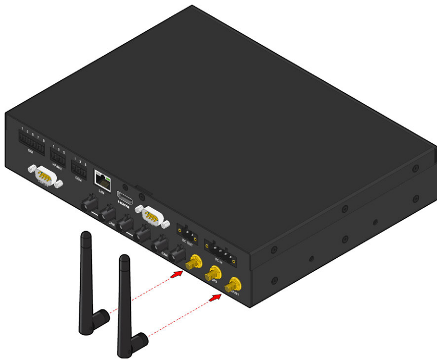
Figure 23: Installing the Wi-Fi/BT antennas
