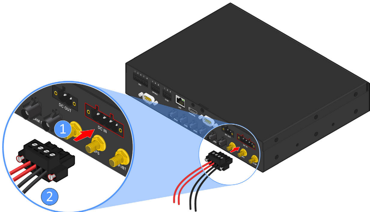
Figure 31: Connecting the Phoenix plug to DC jack
