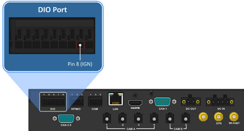
Figure 28: DIO port's pin 8
