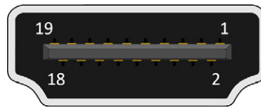
Figure 7: HDMI port diagram
