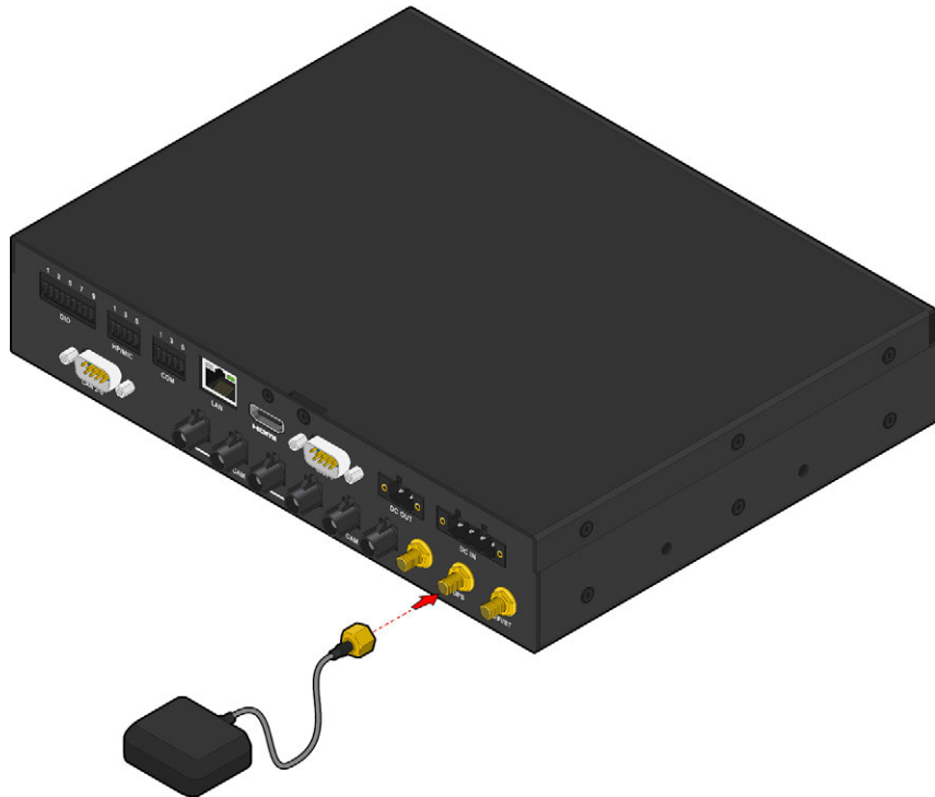
Figure 24: Installing the GPS antenna
