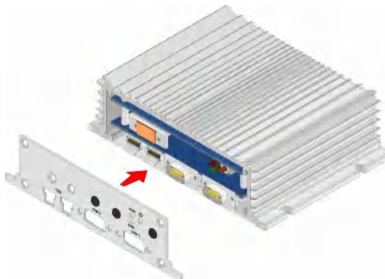
Figure 40: Reinstalling the front panel plate
