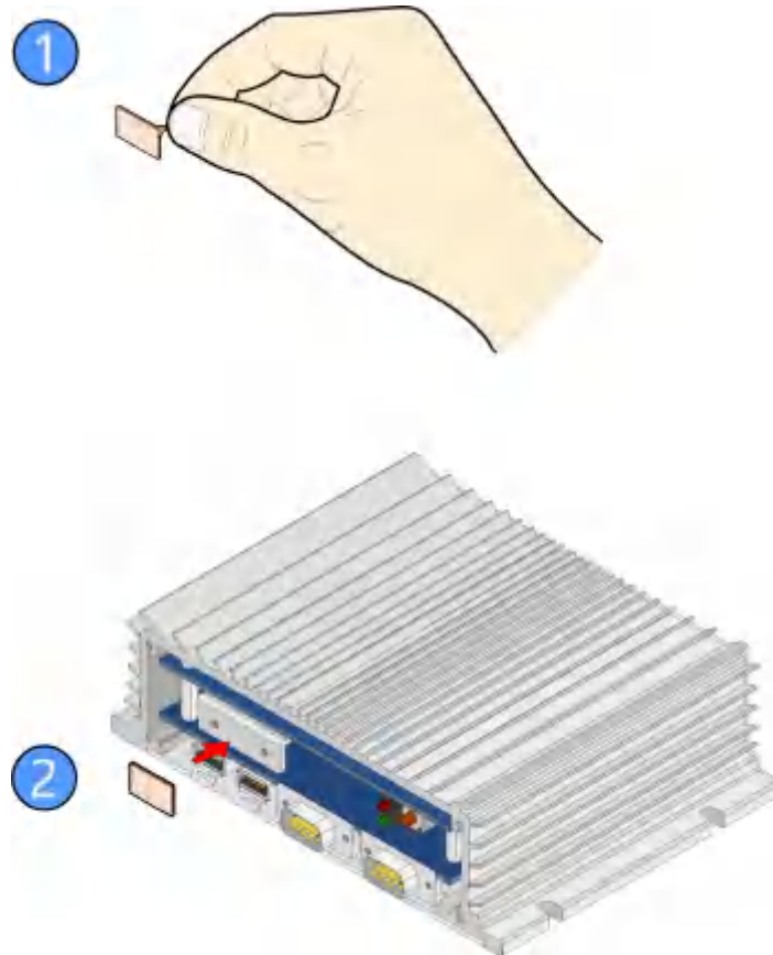
Figure 39: Installing the mSATA heatsink thermal pad
